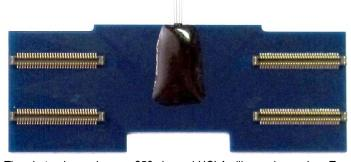
The photo above shows a 256 channel UCLA silicon microprobe. Two RHD 128-channel headstages may be connected to this probe (one on either side) to fully instrument all 256 recording sites.
