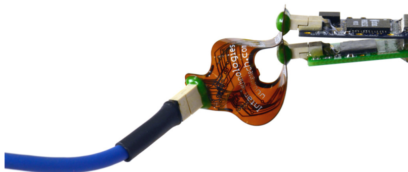
Figure 4. A 96-channel headstage with accelerometer created by combining an RHD2164 amplifier board with an RHD2132 amplifier/accelerometer board.
