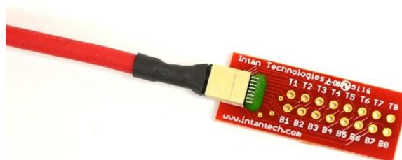
Figure 10. RHS Stim SPI cable adapter circuit board available from Intan Technologies.
