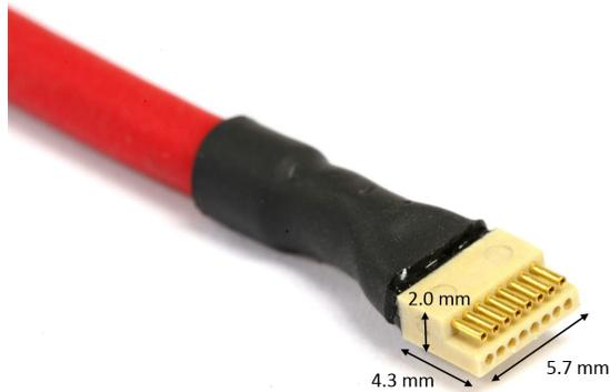
**Figure 1.** Dimensions of a RHS Stim SPI connector from Intan Technologies. The connector on each end is a self-aligning 16-pin Omnetics PZN-16 polarized nano connector.
