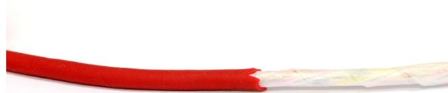
**Figure 2.** Standard cable with red TPE jacket removed. This reduces the cable diameter to 2.4 mm and increases flexibility somewhat.
