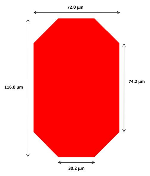
Minimum bond pad pitch (center to center) on RHD2164: 101.6  $\mu$ m (4.000 mil)
