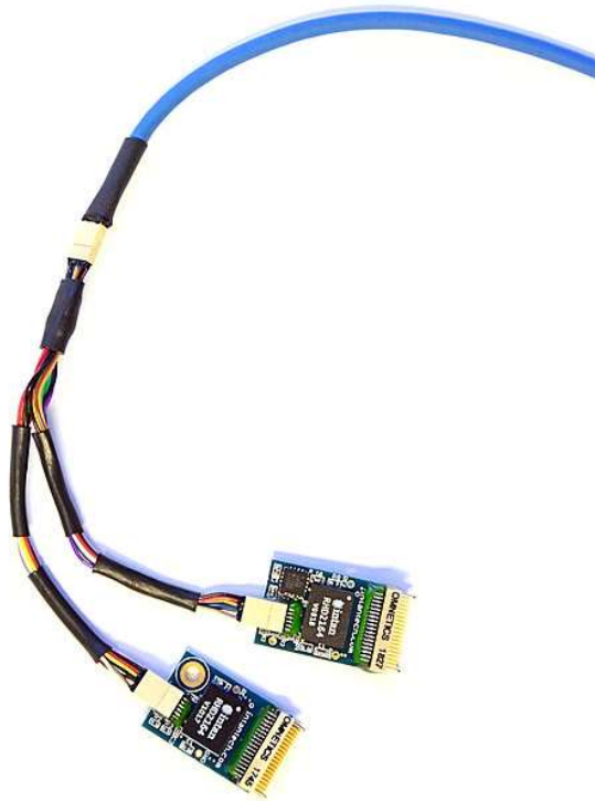
Figure 2. Two RHD2164 amplifier boards (one with an accelerometer) attached to a cable-style dual headstage adapter to create a 128-channel module using a single SPI interface cable.
