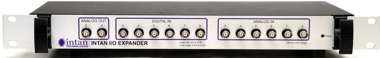
The front panel of the Intan I/O expander provides auxiliary digital and analog inputs, and analog outputs. From left to right:
