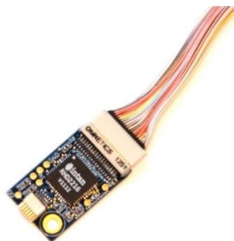
**Figure 9.** Wire adapter plugged into headstage.
