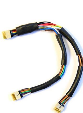
**Figure 21.** RHD dual headstage adapter.
