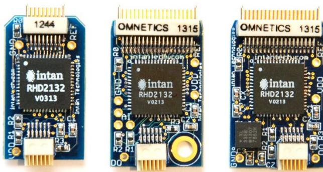
**Figure 14.** Size comparison of RHD 16-channel headstage (left), RHD 32-channel headstage (center), and RHD 32-channel headstage with 3-axis accelerometer (right).
