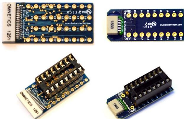
**Figure 8.** 36-pin electrode adapter board (upper left); with 16-pin DIP socket (lower left). 18-pin electrode adapter board (upper right); with 16-pin DIP socket (lower right).
