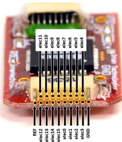
**Figure 6.** Electrode connector pin diagram for 16-channel stim/record headstage.
