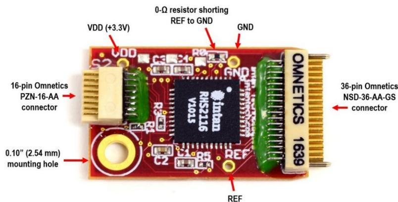
**Figure 5.** 32-channel stim/record headstage with connection ports labeled. The 0-Ω resistor may be removed to disconnect the reference electrode (REF) from ground (GND).
