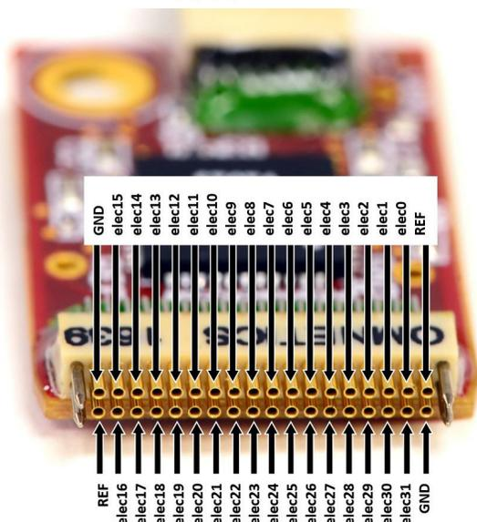
**Figure 7.** Electrode connector pin diagram for 32-channel stim/record headstage.
