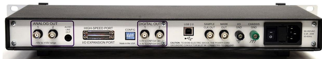
Figure 1B. Intan Stimulation/Recording Controller rear panel.
