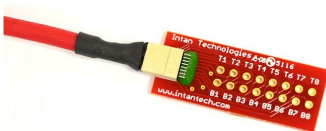
**Figure 11.** Stim SPI cable adapter board plugged into RHS Stim SPI interface cable.
