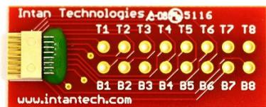
**Figure 10.** Stim SPI cable adapter board
